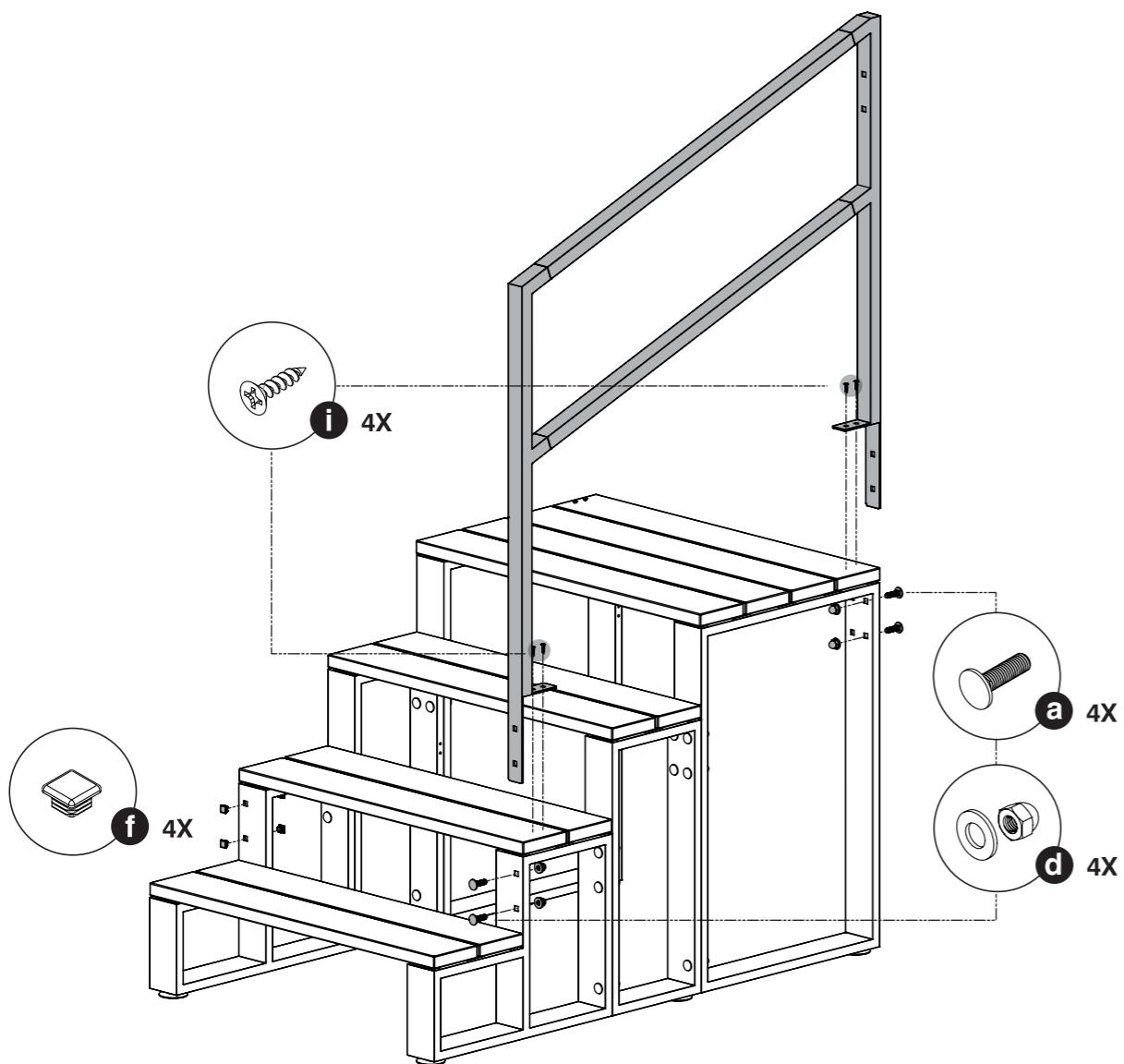
Fix the handrail to the steps on the desired side. Screw at the front of the second step and at the back of the top step with screws, washer and nuts (a-d). DON'T OVER TIGHTEN NUTS.
