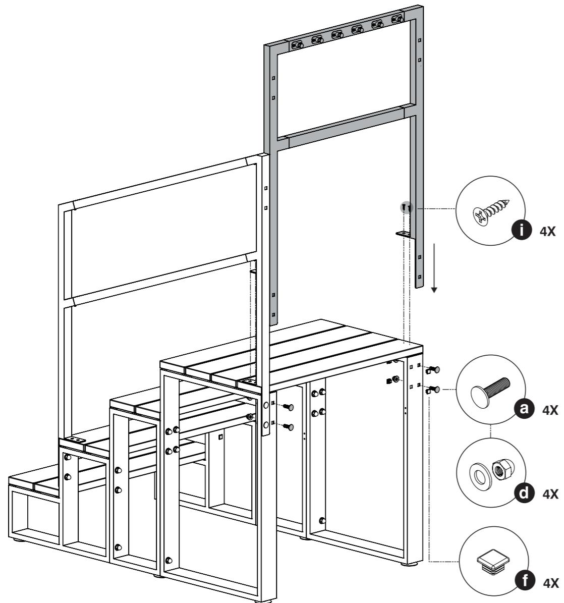
Fix the back handrail to the steps. First at the back with screws, washers and nuts (a-d).
