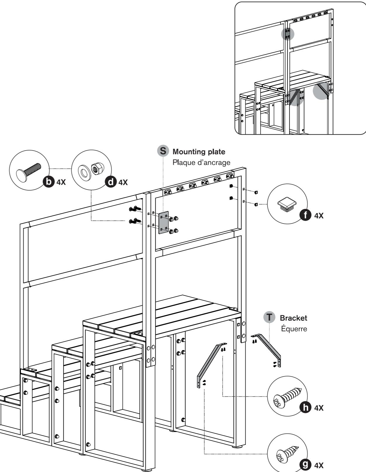
**Fix both handrails together using the mounting plate (S), the screws, washers and the nuts (b-d). DON'T OVER TIGHTEN NUTS.**
