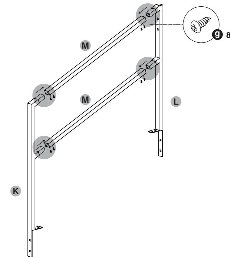
Assemble the side handrail with parts (K-L-M) and screws (g).
