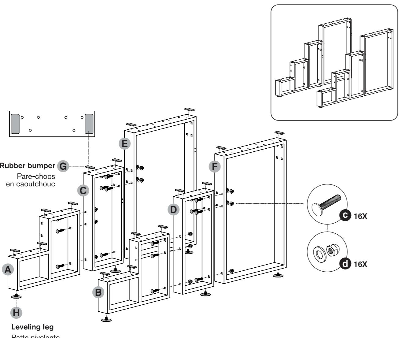
**Assemble parts (A-C-E) and (B-D-F) with screws, washers and nuts (c-d). DON'T OVER TIGHTEN NUTS.**
