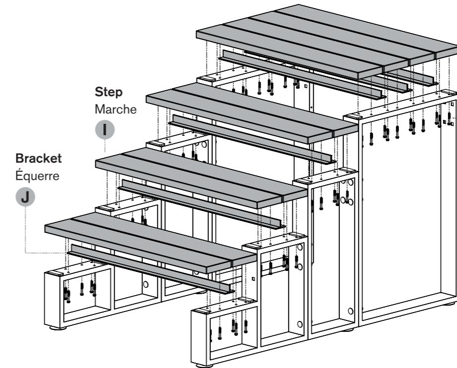
Fix the 6 brackets (J), then the 10 steps (I) with screws and washers (e). DO NOT OVER TIGHTEN SCREWS.
